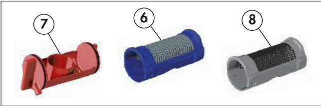
The strainer supplied (blue colour) is composed of a metal mesh with filtration capacity such as to entrap particles of diameter greater than 0,3 mm. This specific strainer mesh is able to intercept all particles remaining in circulation, thereby ensuring optimal initial cleaning of the pipes. After shutting off and draining the DIRTMAGPLUS® device, the strainer (6) can be easily inspected as follows:
