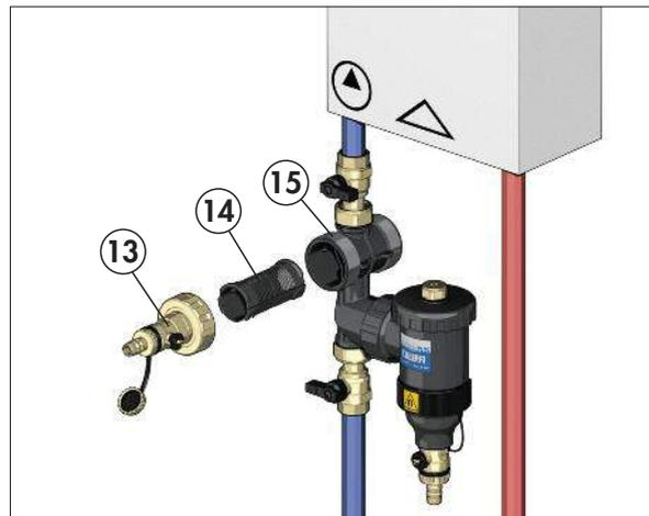
The accessory kit for filling and flushing the circuit (code F49476) is composed of a plug with a drain cock (13) and a black coloured element (14) to be inserted in the strainer container (15) to separate the flows.
